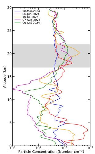
Fig. 2.63. Particle number concentration profiles at standard temperature and pressure (STP; number STP cm<sup>-3</sup>) from the Portable Optical Particle Spectrometer (POPS) aboard the NOAA Global Monitoring Laboratory balloon platform launched from Hilo, Hawaii, ~60 km east of Mauna Loa. The shaded area highlights lower-stratosphere (LS) aerosol signals in Jun, Jul, Aug, and Oct 2024 that arose from the Ruang eruptions in Apr 2024.
