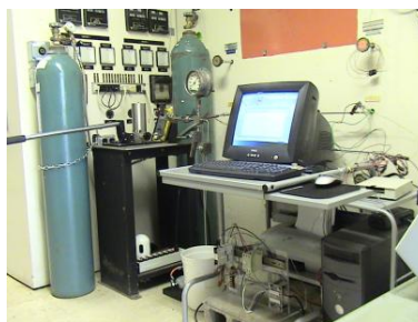
High Pressure and Temperature Flammability Test Set-up in the Pressure Barricade Cell Area
