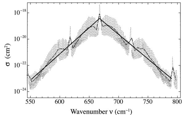
Fig. 1. Absorption cross-section, in  $\text{cm}^2$ , for a CO<sub>2</sub> molecule as a function of frequency around  $15 \mu\text{m}$  wavelength (light gray dotted curve); note the logarithmic scale. Also shown are a “coarse grained” spectrum (medium gray dashed curve) obtained by averaging over intervals of width  $5 \text{ cm}^{-1}$ , and a drastically simplified version (black, solid line) that we use for the analytical order-of-magnitude estimates.
