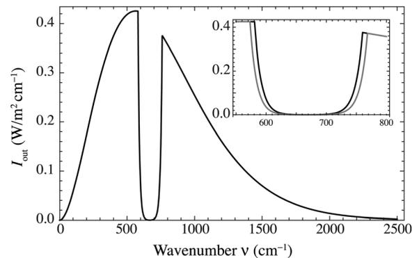
Fig. 2. The transmitted intensity through the atmosphere as a function of frequency, as given by  $(1 - P_{\text{return}})B(\nu, T)$ , for  $T = 288 \text{ K}$ , using the triangular approximation (8) to the  $\text{CO}_2$  absorption spectrum in Eq. (13). Inset: detail of the region between  $550$  and  $800 \text{ cm}^{-1}$  for the current  $\text{CO}_2$  concentration of 390 ppm (black curve) and for double the concentration, or 780 ppm (gray curve).
