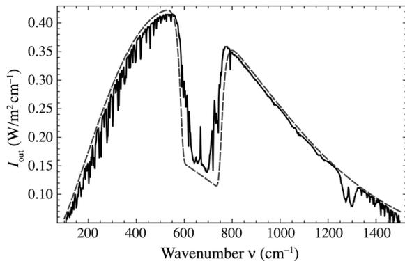
Fig. 4. MODTRAN calculation (black, solid curve), and our approximation (dashed, gray curve); see text for details.
